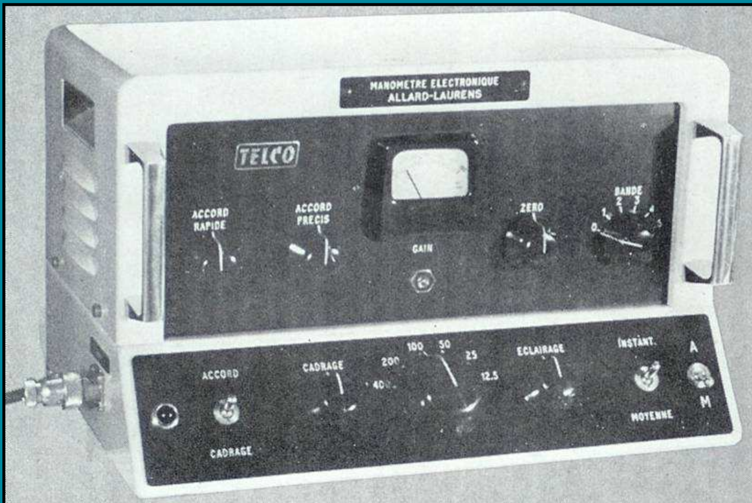
Unit for Allard and Laurens' tip micromanometer
